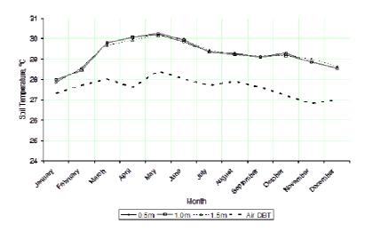
Fig. 5: Average air temperature and soil temperature at 0.5m, 1.0m and 1.5m depths underground
